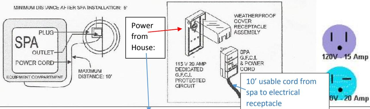
**This MUST be a dedicated electrical line—the only item drawing or using electrical power on this line. ANY shared line will not run the hot tub!**
